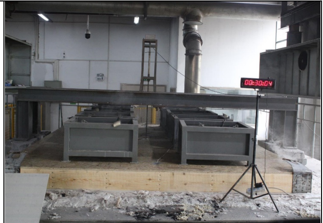
Photo 18: The unexposed face of sample (After test duration of 30 minutes)
