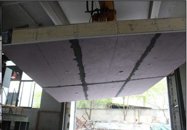
Photo 14: The exposed face before the test
