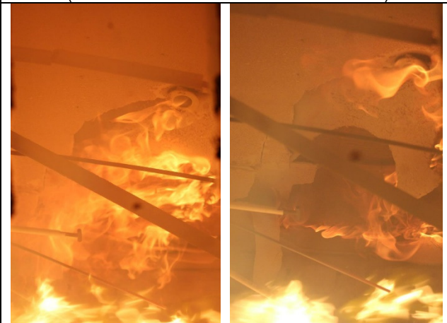
Photo 23: The exposed face of sample (After test duration of 70 & 80 minutes)
