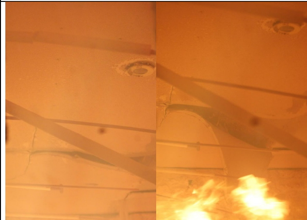
Photo 19: The exposed face of sample (After test duration of 30 & 40 minutes)
