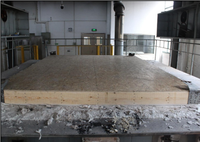
Photo 13: The unexposed face before the test
