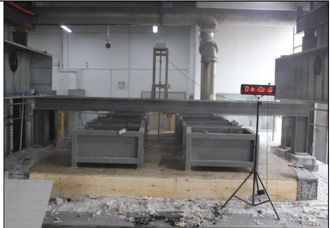
Photo 22: The unexposed face of sample (After test duration of 70 minutes)
