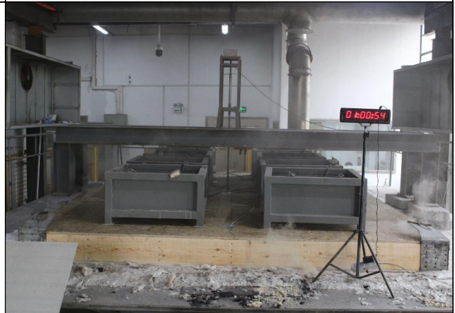
Photo 20: The unexposed face of sample (After test duration of 60 minutes)
